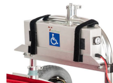
Auxiliary Battery Tray
