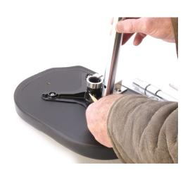
3.) Remove the old (short) seat post and insert the new (longer) seat post, and align the hole with the threaded set screw hole.
