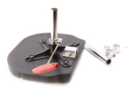
1.) Loosen (don't remove) the bolt on the fixed clamp.
