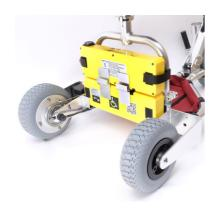
2.) Insert the second battery and align with the first, with the wire pigtail towards the LOWER left. This way the batteries do not need to swap positions to connect to the scooter. Secure the upper battery to the yoke with the hook-Velcro strips.
