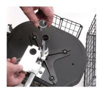
3.) Remove the seat from the yoke and set it upside down. Slide the 3cm long (approx.. 1 1/8 inch) seat spacer over the seat post. Now slide the flat metal hook plate over the seat post with the hooks pointing towards the bottom of the seat, followed by the 2cm (3/4 inch) spacer. These parts may be secured from falling off during seat removal using tape or adhesive.
